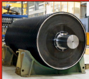
Conveyor Head Pully
